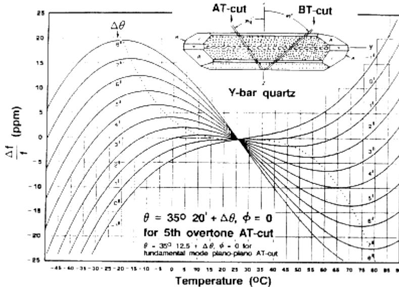
To further minimize temperature related frequency changes, quartz sensors are placed in water-cooled housings, with the cooling water set at 20°C. In theory, this configuration results in the frequency-temperature behavior being minimized or even eliminated. In practice, however, this is not realized and worse, the process engineer is not even aware that it is a factor.
